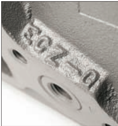
The head casting numbers are located under the lip of the intake ports. ECZ-G and 113 heads are the most sought after.
